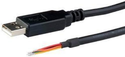
The TTL-232R-3V3-WE ("wire ended") is a USB to Serial (TTL level) converter cable which allows for a simple way to connect TTL interface devices to USB. This version of FTDI's USB to TTL serial adapter cable has its I/O pins configured to operate at 3.3V levels.
