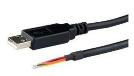
The TTL-232R-5V-WE ("wire ended") is a USB to Serial (TTL level) converter cable which allows for a simple way to connect TTL interface devices to USB. This version of FTDI's USB to TTL serial adapter cable has it's I/O pins configured to operate at 5V levels.
